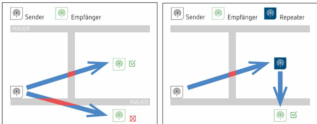
Wall or ceiling thickness effective for attenuation
