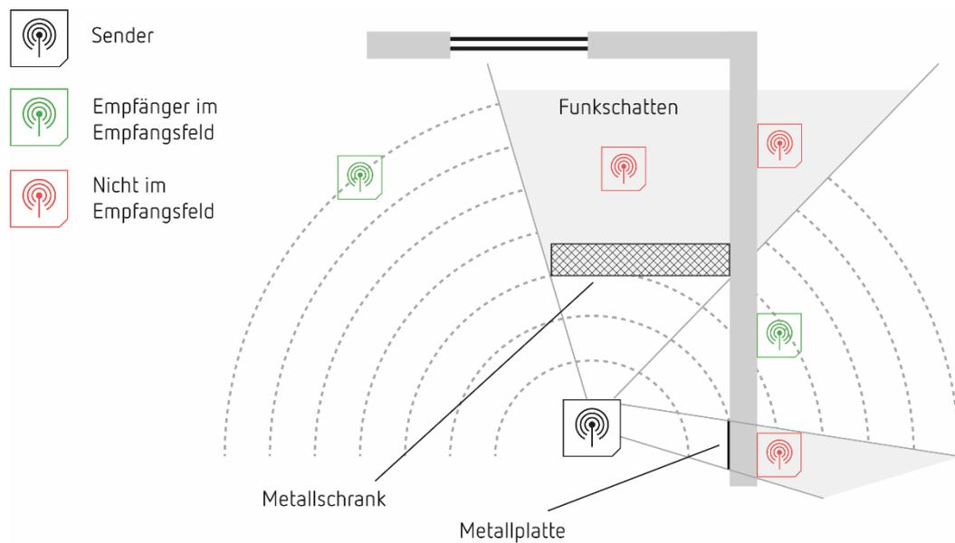
Radio shadow e.g. due to metal parts
