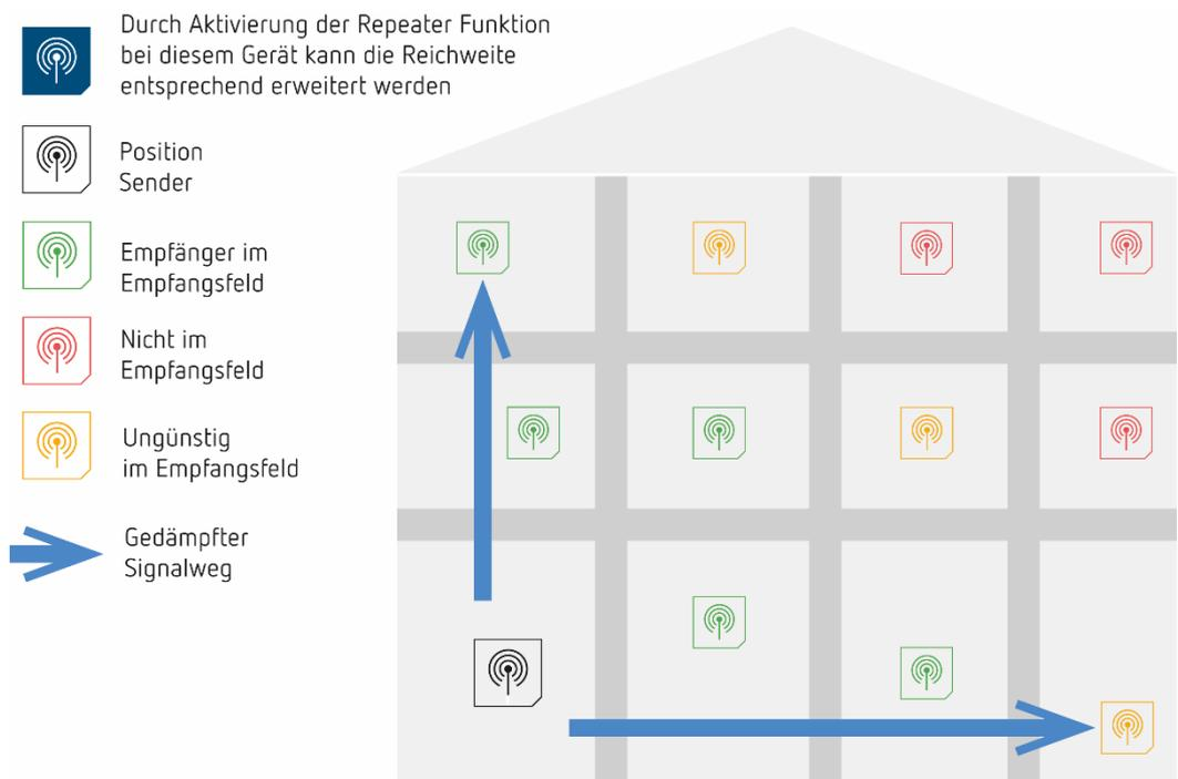
Example with activated repeater function with a Theben KNX-RF actuator
