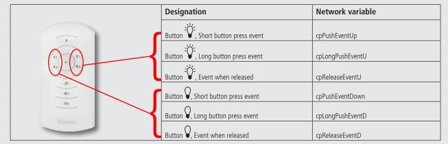
IR group addresses I and II are allocated permanently to 4 buttons on theSenda S user remote control, and cannot be changed. Further information can be found in the operating instructions of theSenda S.
