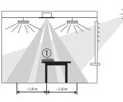
In every case it is recommended to perform the calibration with a mix of approximately 50% each of artificial light and daylight. When the detector is powering up, calibration may only be performed after the start-up phase has ended. During the start-up phase the LED of the detector flashes in one second intervals.
